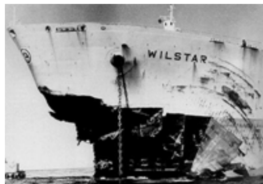
Bow damage caused by a giant wave
